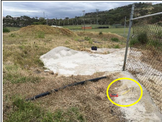
Photo 9. Hand-held Temperature Probe - Surface (300mm depth) - 17 th November 2017 - internal northern fence line
