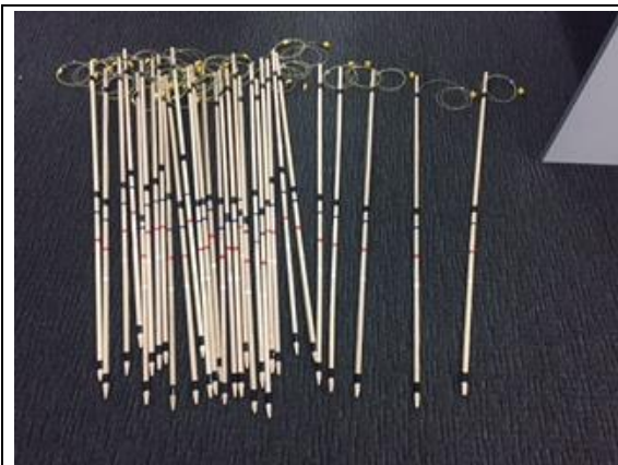
Photo 19. Manufacture of permanent Temperature Probe - (500mm depth) - 2 nd -10 th January 2018
