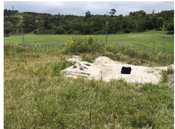
Photo 22. Four (4) metre grid pattern of permanent Temperature Probe - (500mm depth) - 28 th January 2018
