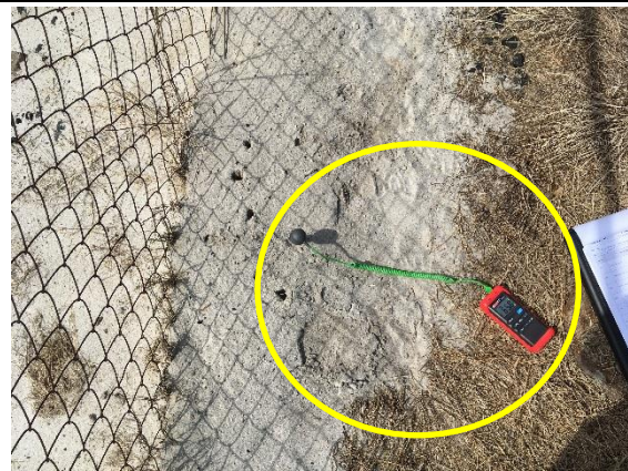
Photo 10. Hand-held Temperature Probe - Surface (150mm depth) - 24 th November 2017 - internal northern fence line
