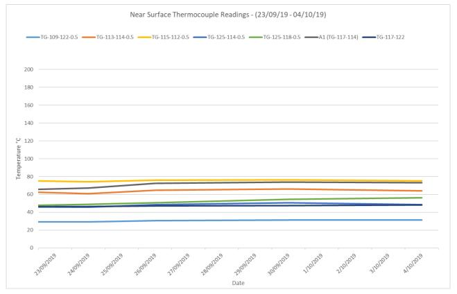
The near-surface temperature at selected points across the northwest hotspot over the period of monitoring appear to remain consistent.
