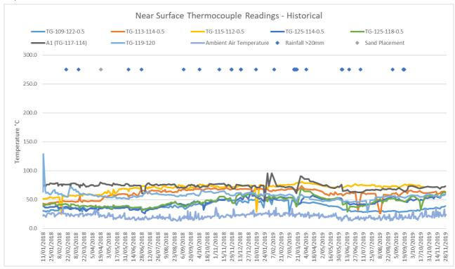
The near surface temperature appears to be trending downwards following the placement of sand (approximately 100mm) across the surface of the northwest hotspot grid monitoring area.
