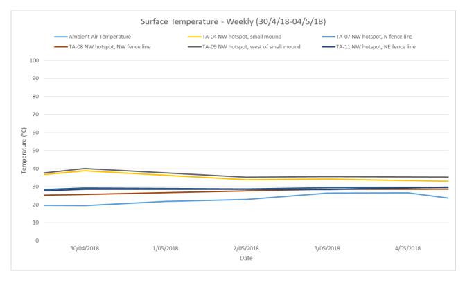
The surface temperature at selected points across the northwest hotspot over the week of monitoring -30/4/2018 to 04/5/2018, appear to remain consistent.
