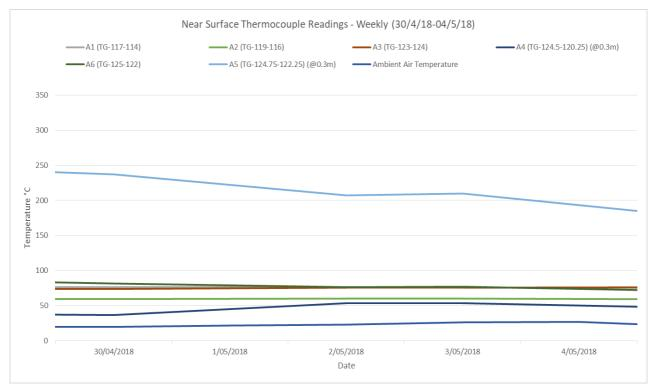
The near surface temperature at selected points across the northwest hotspot over the week of monitoring -30/4/2018 to 04/5/2018, appear to remain consistent.
