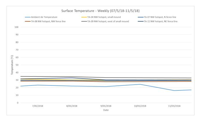
The surface temperature at selected points across the northwest hotspot over the week of monitoring -07/5/2018 to 11/5/2018, appear to remain consistent.
