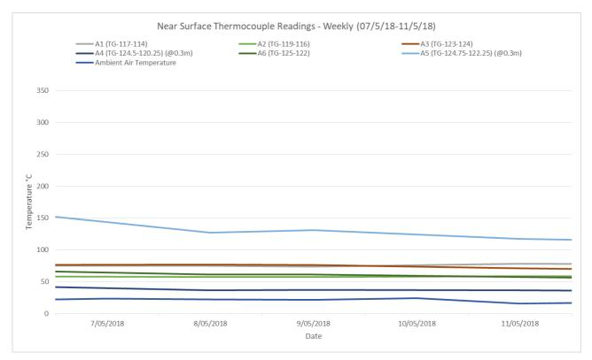
The near surface temperature at selected points across the northwest hotspot over the week of monitoring -07/5/2018 to 11/5/2018, appear to remain consistent.
