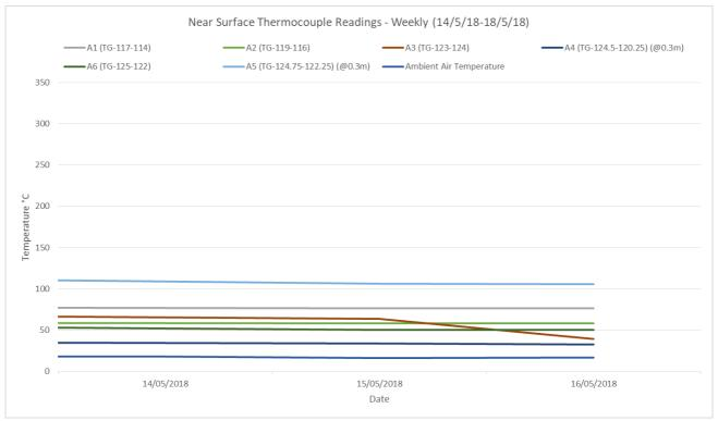
The near surface temperature at selected points across the northwest hotspot over the week of monitoring -14/5/2018 to 18/5/2018, appear to remain consistent.
