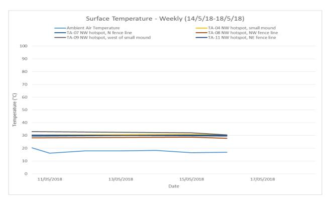
The surface temperature at selected points across the northwest hotspot over the week of monitoring -14/5/2018 to 18/5/2018, appear to remain consistent.
