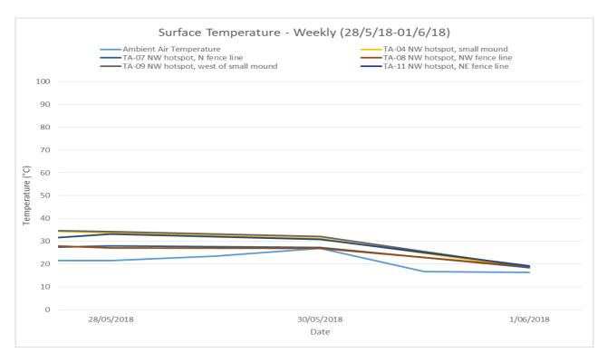
The surface temperature at selected points across the northwest hotspot over the week of monitoring -28/5/2018 to 01/6/2018, appear to remain consistent.
