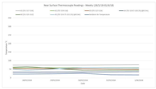
The near surface temperature at selected points across the northwest hotspot over the week of monitoring -28/5/2018 to 01/6/2018, appear to remain consistent.
