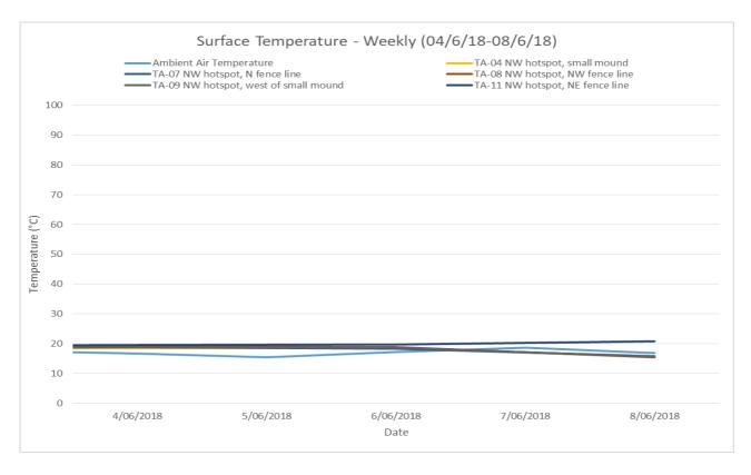
The surface temperature at selected points across the northwest hotspot over the week of monitoring -04/6/2018 to 08/6/2018, appear to remain consistent.
