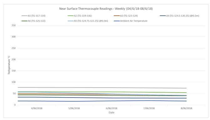
The near surface temperature at selected points across the northwest hotspot over the week of monitoring -04/6/2018 to 08/6/2018, appear to remain consistent.
