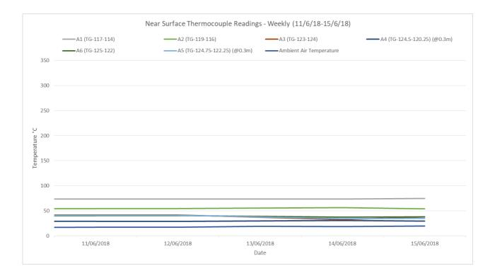
The near surface temperature at selected points across the northwest hotspot over the week of monitoring -11/6/2018 to 15/6/2018, appear to remain consistent.
