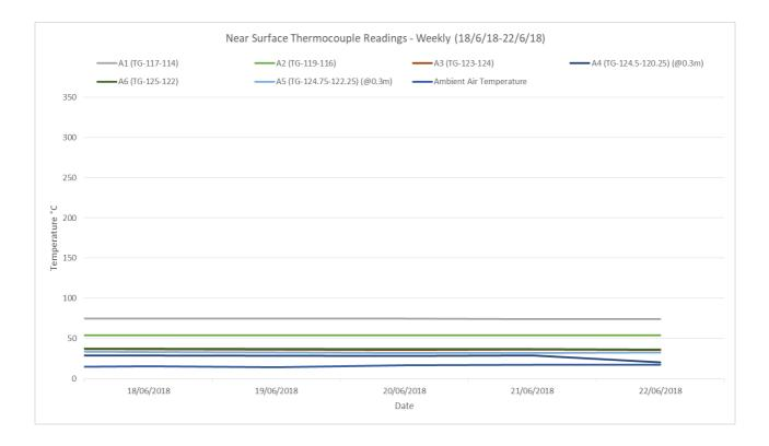
The near surface temperature at selected points across the northwest hotspot over the week of monitoring -18/6/2018 to 22/6/2018, appear to remain consistent.
