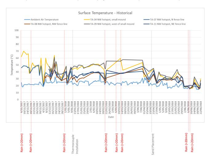
The surface temperature appears to have decreased and stabilised following the placement of sand (approximately 100mm) across the surface of the northwest hotspot grid monitoring area.
