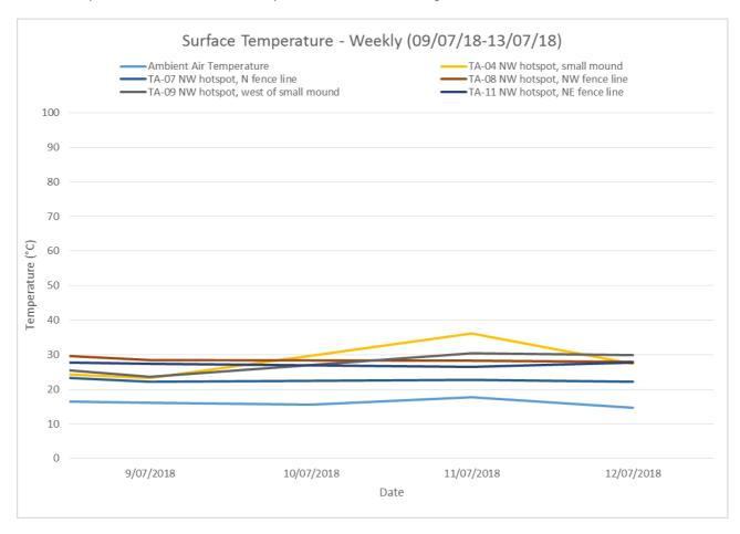
The surface temperature at selected points across the northwest hotspot over the week of monitoring -09/07/2018 to 13/07/2018, appear to remain consistent.
