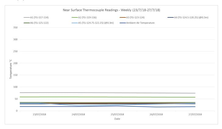
The near surface temperature at selected points across the northwest hotspot over the week of monitoring -23/07/2018 to 27/07/2018, appear to remain consistent.
