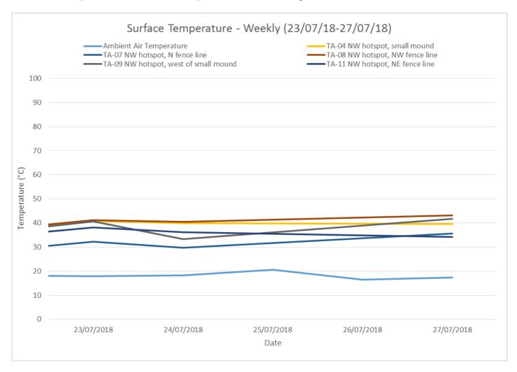
The surface temperature at selected points across the northwest hotspot over the week of monitoring -23/07/2018 to 27/07/2018, appear to remain consistent.
