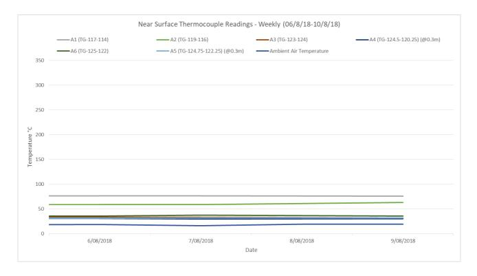
The near surface temperature at selected points across the northwest hotspot over the week of monitoring -06/08/2018 to 10/08/2018, appear to remain consistent.
