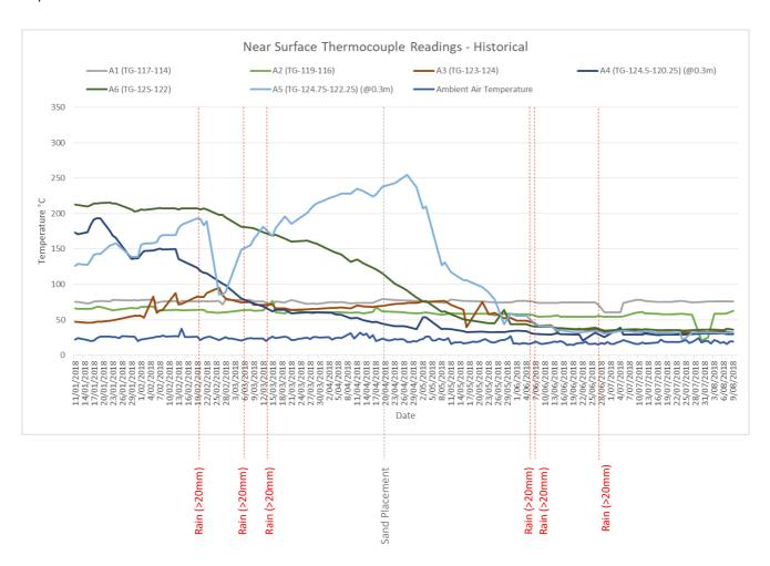
The near surface temperature appears to be trending downwards following the placement of sand (approximately 100mm) across the surface of the northwest hotspot grid monitoring area.
