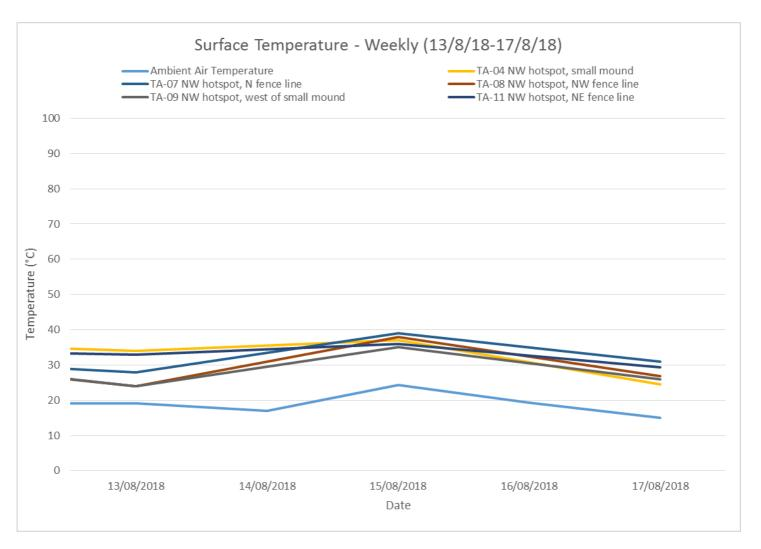
The surface temperature at selected points across the northwest hotspot over the week of monitoring -13/08/2018 to 17/08/2018, appear to remain consistent.
