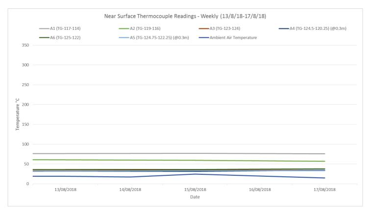
The near surface temperature at selected points across the northwest hotspot over the week of monitoring - 13/08/2018 to 17/08/2018, appear to remain consistent.
