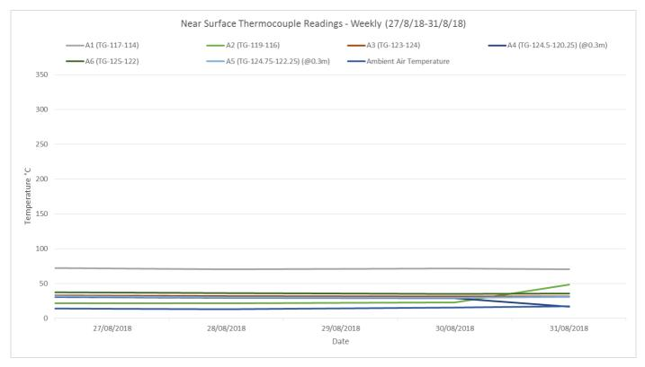
The near surface temperature at selected points across the northwest hotspot over the week of monitoring – 27/08/2018 to 31/08/2018, appear to remain consistent.
