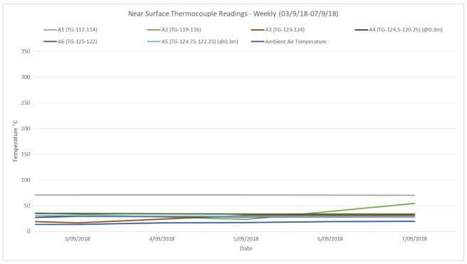
The near surface temperature at selected points across the northwest hotspot over the week of monitoring – 03/09/2018 to 07/09/2018, appear to remain consistent.
