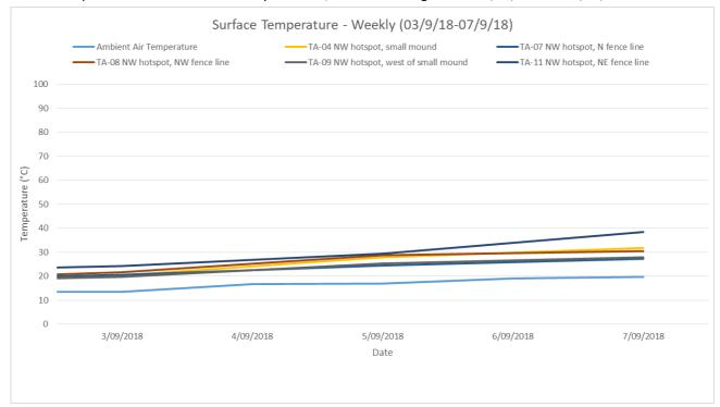
The surface temperature at selected points across the northwest hotspot over the week of monitoring -03/09/2018 to 07/09/2018, appear to remain consistent.
