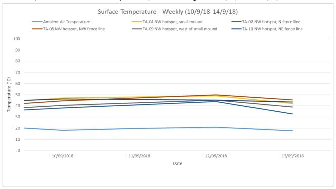
The surface temperature at selected points across the northwest hotspot over the week of monitoring -10/09/2018 to 14/09/2018, appear to remain consistent.
