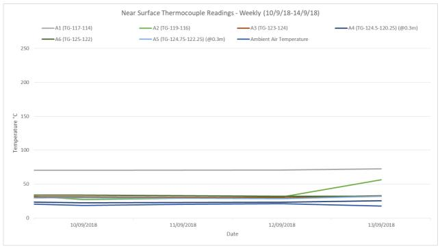
The near surface temperature at selected points across the northwest hotspot over the week of monitoring -10/09/2018 to 14/09/2018, appear to remain consistent.
