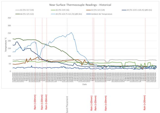
The near surface temperature appears to be trending downwards following the placement of sand (approximately 100mm) across the surface of the northwest hotspot grid monitoring area.
