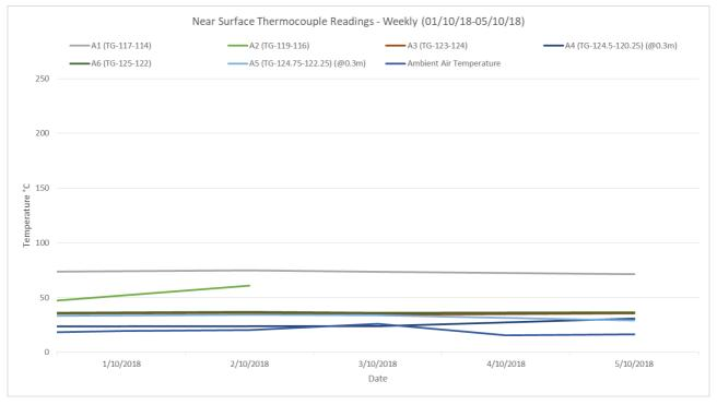
The near surface temperature at selected points across the northwest hotspot over the week of monitoring - 01/10/2018 to 05/10/2018, appear to remain consistent.
