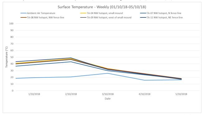
The surface temperature at selected points across the northwest hotspot over the week of monitoring -01/10/2018 to 05/10/2018, appear to remain consistent.
