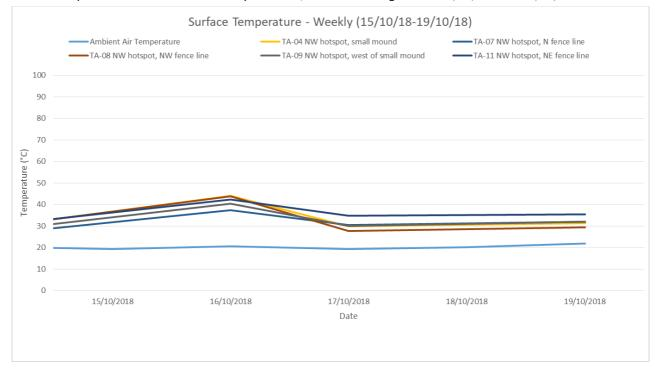
The surface temperature at selected points across the northwest hotspot over the week of monitoring -15/10/2018 to 19/10/2018, appear to remain consistent.
