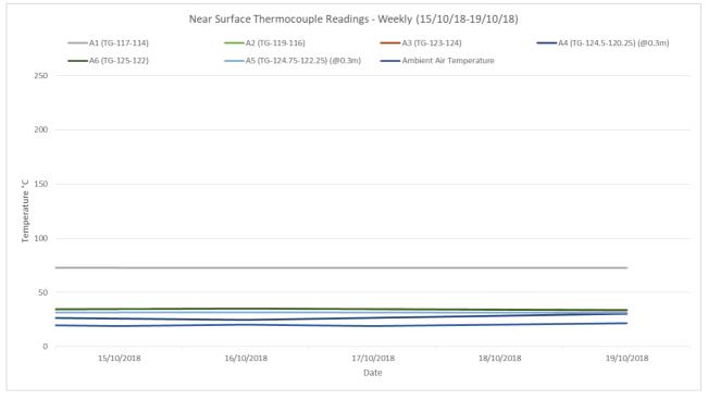
The near surface temperature at selected points across the northwest hotspot over the week of monitoring -15/10/2018 to 19/10/2018, appear to remain consistent.
