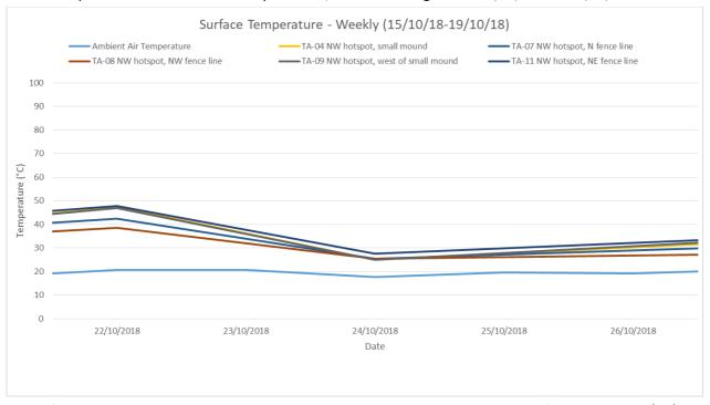
The surface temperature at selected points across the northwest hotspot over the week of monitoring -22/10/2018 to 26/10/2018, appear to remain consistent.
