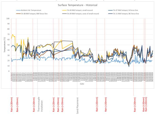
The surface temperature appears to have decreased and stabilised following the placement of sand (approximately 100mm) across the surface of the northwest hotspot grid monitoring area.
