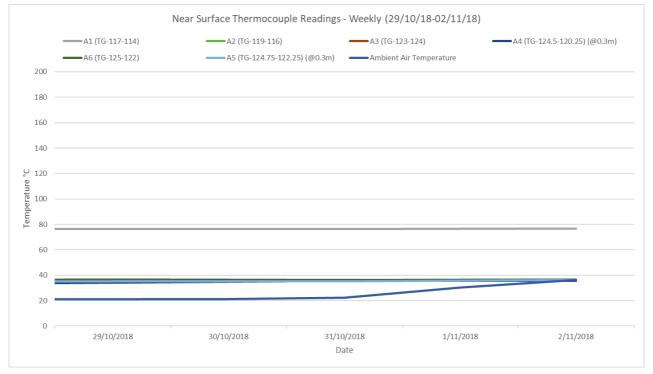
The near surface temperature at selected points across the northwest hotspot over the week of monitoring -29/10/2018 to 02/11/2018, appear to remain consistent.
