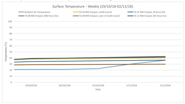
The surface temperature at selected points across the northwest hotspot over the week of monitoring -29/10/2018 to 02/11/2018, appear to remain consistent.
