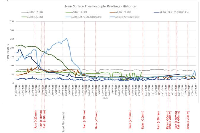
The near surface temperature appears to be trending downwards following the placement of sand (approximately 100mm) across the surface of the northwest hotspot grid monitoring area.
