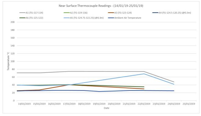
The near surface temperature at selected points across the northwest hotspot over the period of monitoring appear to remain consistent.
