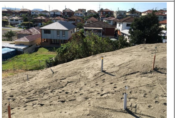
Photo 12. Ongoing near surface temperature monitoring across area of concern - April 2018
