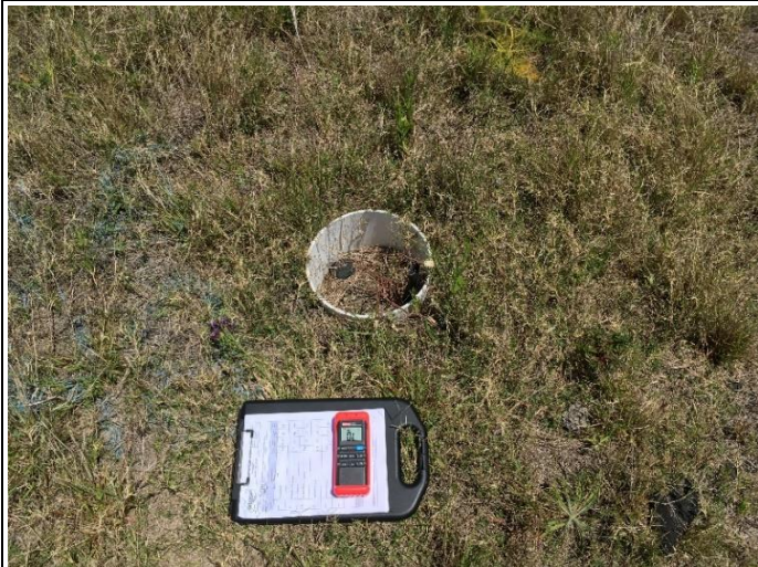
Photo 9. Monitoring of pre-existing Avopiling Thermocouple Wells - Western Playground area
