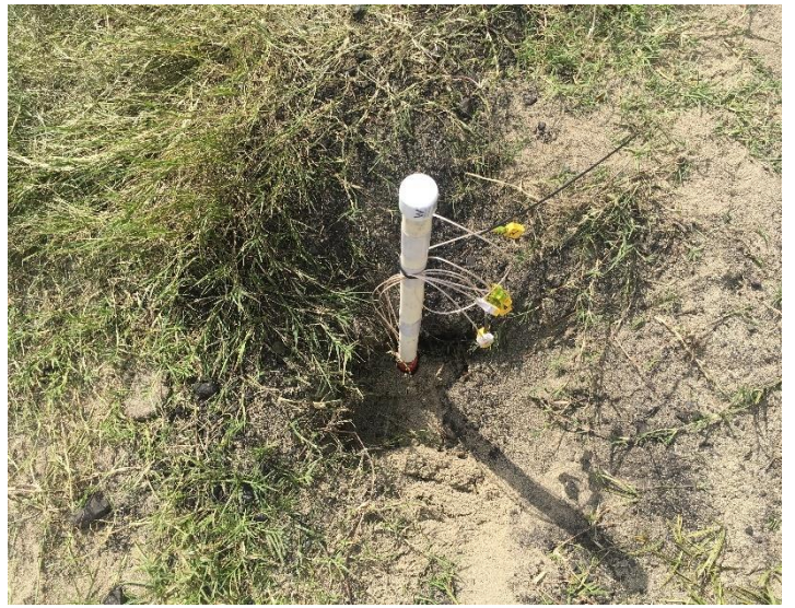
Photo 14. Installation and Monitoring of Subsurface Thermocouples – October 2018
